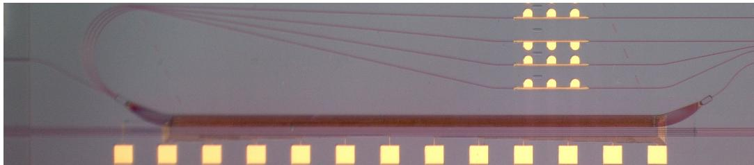
**Figure 3. Photograph of the realized device (size: 1.7x8.2 mm<sup>2</sup>).**
