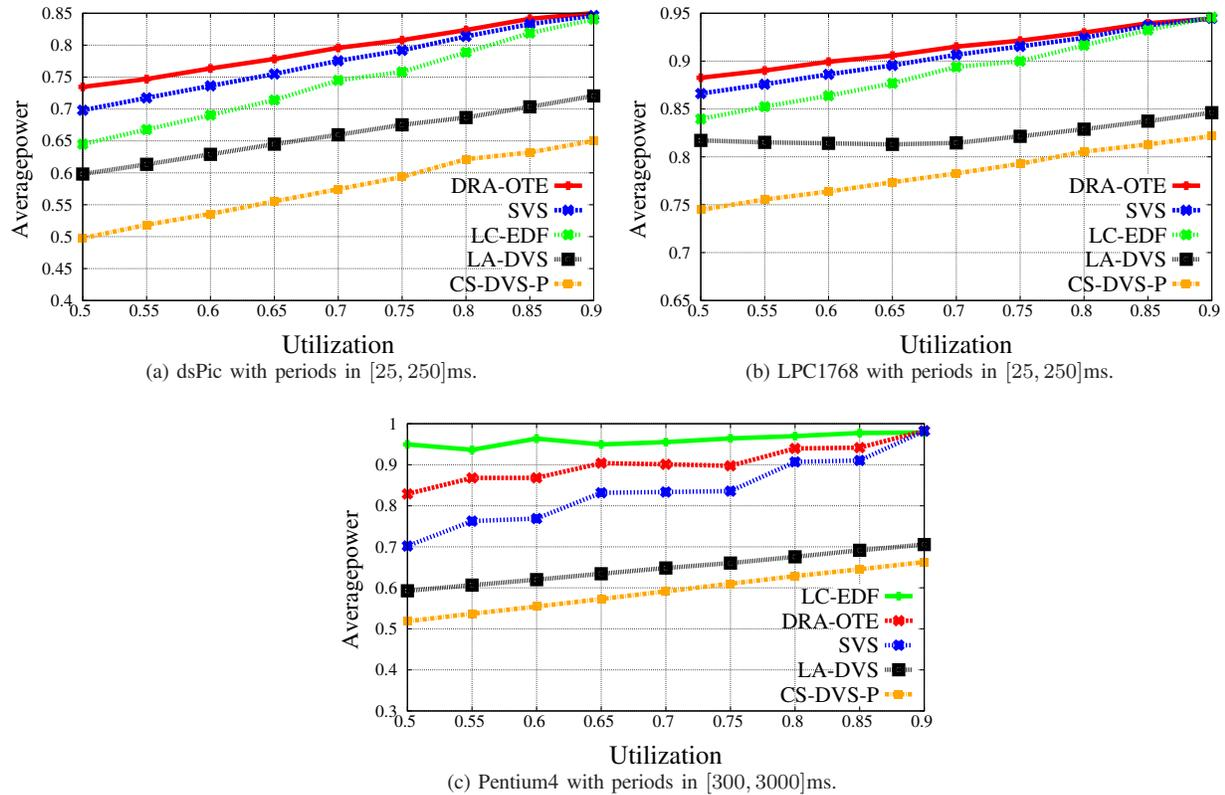
Fig. 4: Average power consumption considering task early terminations.
